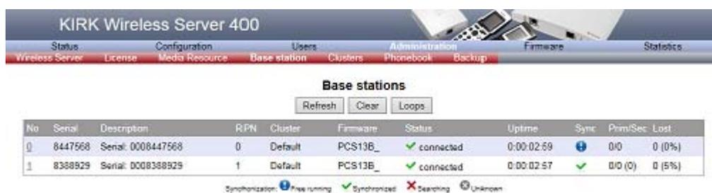
In the example above, there are two bases in the Spectralink IP-DECT Server 400 solution. Base station 1 is Synchronization on base 0 (Zero). Repeaters are not visible in the server, and are add-ons to the system and are not manageable by the system. A repeater is managed directly on the repeater itself using a PC and a repeater programming kit.
